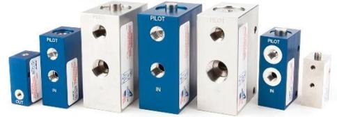
Aladco® Clean-Check® valve is a normally closed check valve that can be overridden by air piloting or manually to allow two-way flow. The tightly sealed Clean-Check® valves are used on pneumatic devices to stop air release when the device is stopped, which prevents drifting of the device and any attached load. Clean-Check® valves are unique in that they can be used in environments that need to stay very clean, but they also can tolerate exposure to external dirt and liquids.
